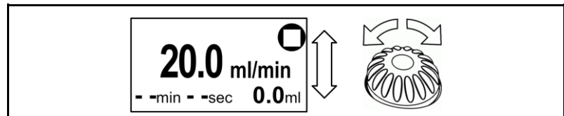
Fig. 26: Moving the operating menu up / down
